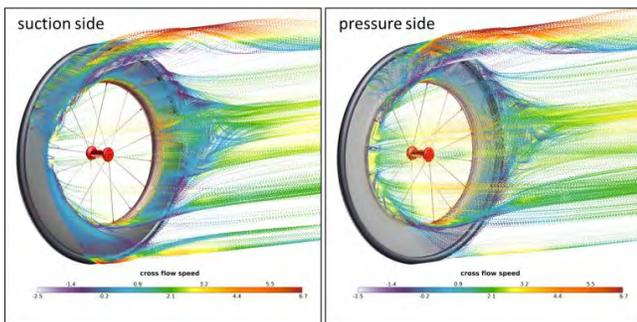
*Streamlines in steady-state flow calculations show cross flow patterns for two different wheel prototypes.*
