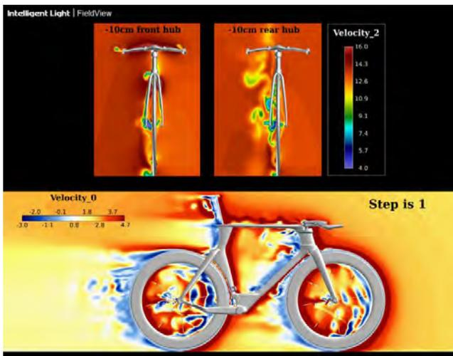
Scott Plasma racing bicycle frame with Zipp Firecrest 808 wheels. DES simulation performed with STAR-CCM+, three cutplanes showing relative air velocity.
