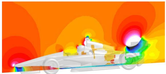
CFD's ability to help analysts understand changes in flow structures and identify the basic aerodynamic properties that cause those changes helps create a knowledge base that informs future projects. Although operating
